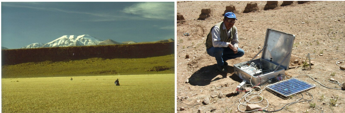
Fig. 4.1: Above left: Fundamental layout in the field (DL: data logger). The probes are in a cross layout. Above right: Connection of the telluric probes at the input of an operational amplifier. Below left: Layout of telluric cables. Below right: View on data logger, electronics for controlling the fluxgate magnetometer, external GPS for time synchronization and solar panel. The instruments should be buried to protect them from the influence of temperature variations.
