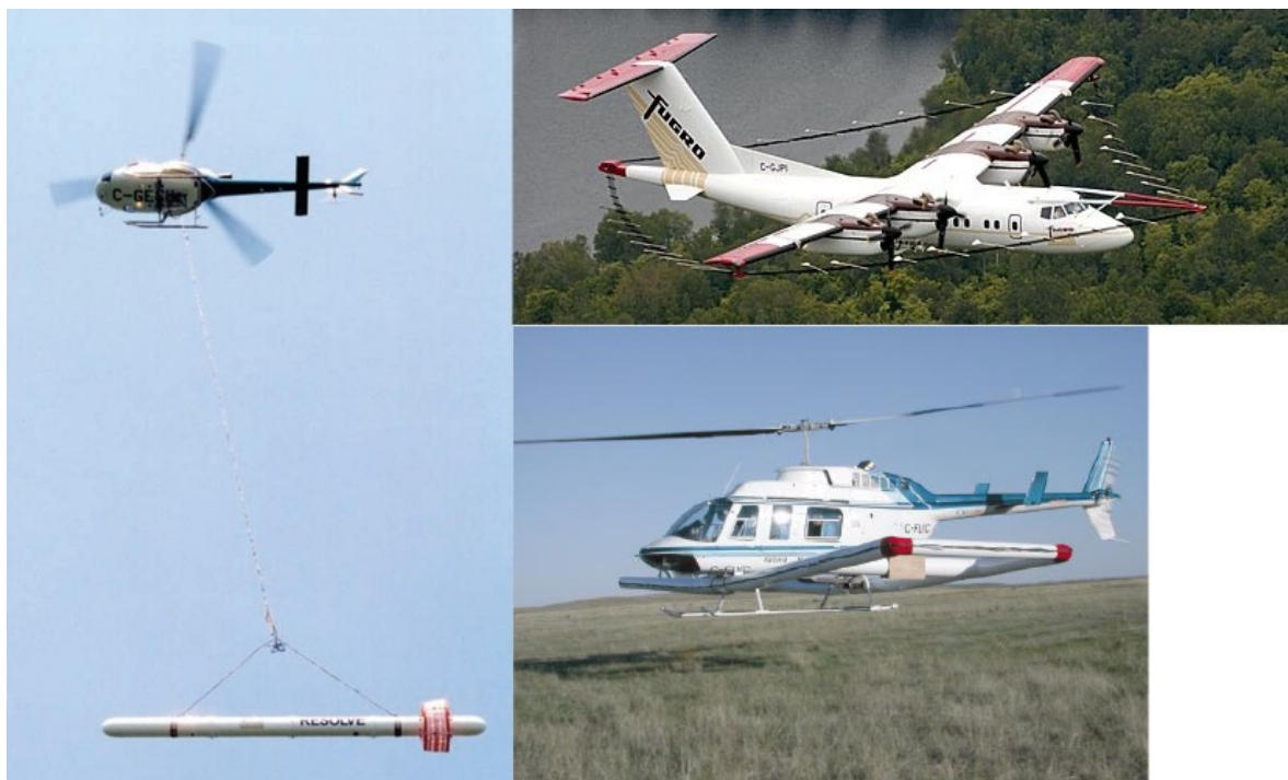
Fig 11.15b: Layout of aero-electromagnetic devices. Links: Bird at a helicopter, right top: TEM-System (Fugro Airborne Surveys, www.fugroairborne.coft.au/index.shtml ), right below: Helicopter-TEM to detect UXO (unexploded – also unexplored – ordnance) (Oak Ridge Airborne Geophysical System, from: Beard et al., Geophysics, 69, 2004).
